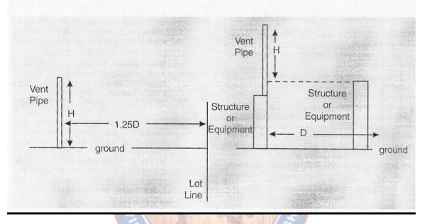
H = Minimum height in feet of vent pipe above the ground or above any structure or equipment within distance (D) where personnel might be present.
