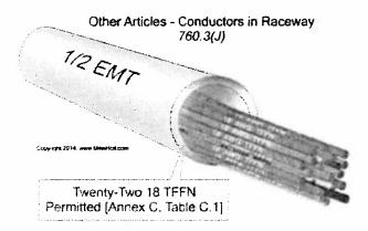
The number and size of conductors or cables in a raceway are limited in accordance with 300.17.
