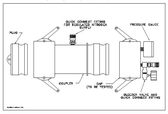
Vapor Coupler Test Assembly. Use a compatible OPW 634-B cap, or equivalent, equipped with a center probe to open the poppet, the appropriate pressure measuring device to monitor the pressure decay, and a connection for the introduction of nitrogen into the system. See Figure 3 for example.
