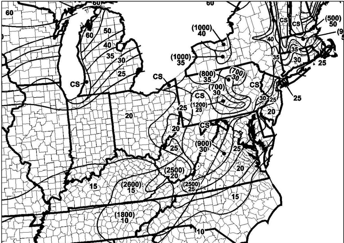
In CS areas, site-specific Case Studies are required to establish ground snow loads. Extreme local variations in ground snow loads in these areas preclude mapping at this scale.
