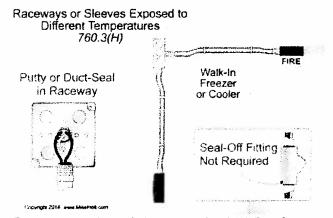
Raceways must be sealed to prevent the circulation of warm air to a colder section of the raceway or sleeve [300.7(A)].
