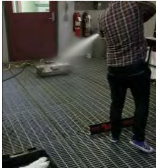
Figure 10: Participant aiming at the base of the BullEx ITS
