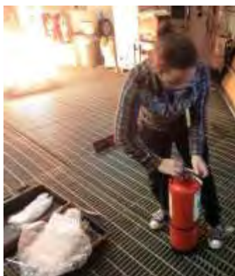
Figure 17: Participant turning back to the fire while attempting to free the pin from the BullEx Smart Extinguisher
