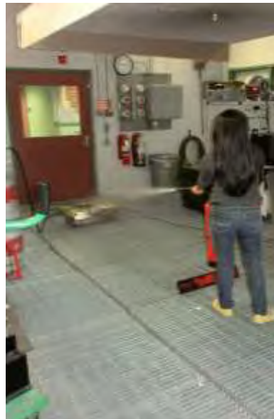
Figure 14: Participant continuously deploys agent on propane fire, thereby preventing re-ignition
